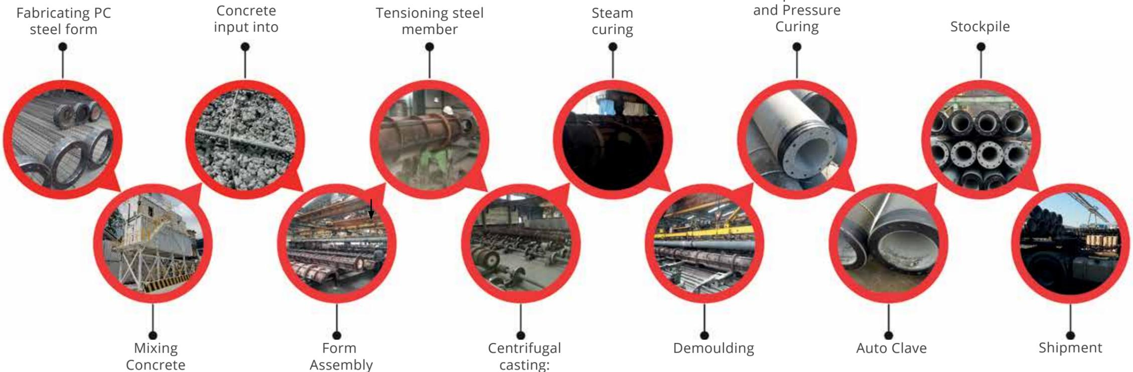
The quality depends on centrifugal force & speed. The pile section is divided into several segregated layers such as laitance, paste, mortar, and concrete layers.
