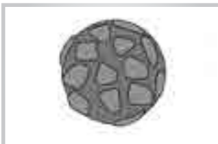
CEMAX adsorbs into small cracks clinker, saturate the charges and reduce the surface energy forces
